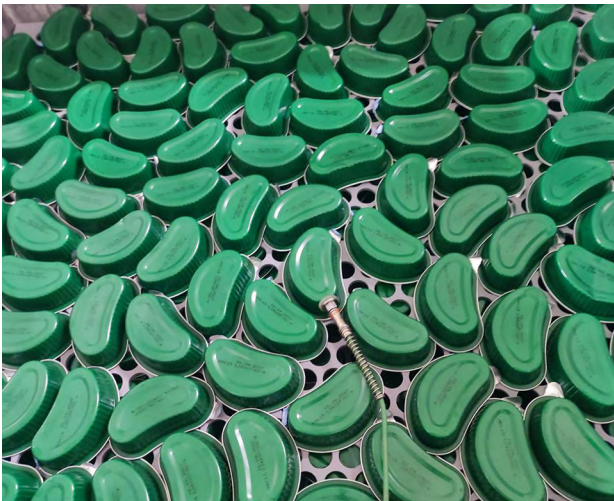
Figure 5. Thermocouple probe placed in the thermal centre of a tuna pâté can
