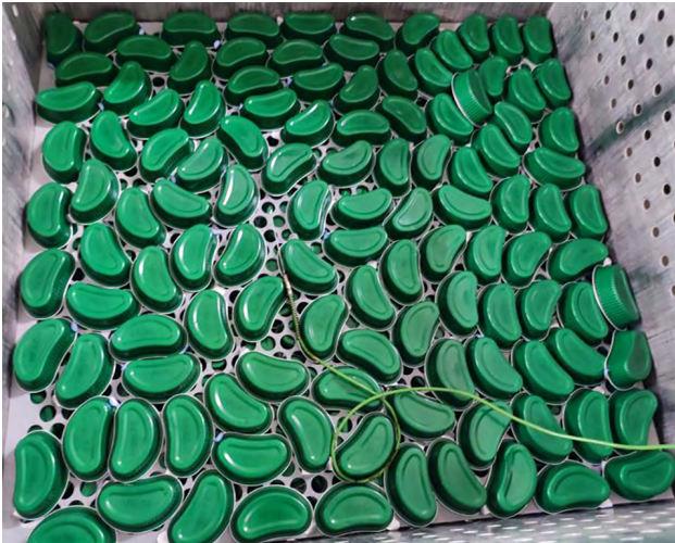
Figure 4. Thermocouple probes placed outside the tuna pâté cans in the carts
