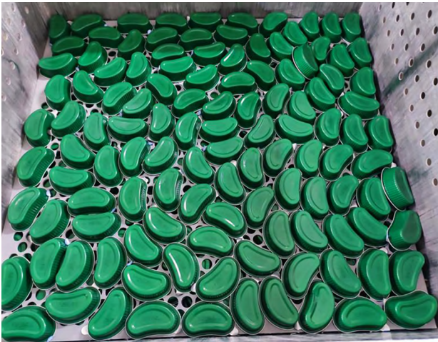
Figure 3. Tuna pâté cans of 60 g positioned in a cart and ready for thermal processing
